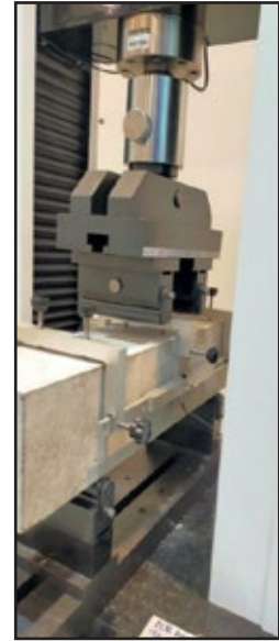
ASTM C1609 Setup
